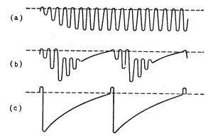
Fig. 2. (a) Start of oscillations in sine-wave oscillator in circuit very similar to Fig. I except for closeness of coupling. (b) Squegging condition obtained by increasing the coupling slightly. (c) Alleged result of tightening coupling to the limit.
