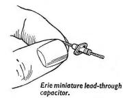
BS415-1957 and is made in five sizes with capacitances of from 470 pF to 20 kpF. The latter is for earth leads only. Another "aerial isolator". but of tubular ceramic form with side-entry wires, was shown by Stability Capacitors. It measures 0.7 in long, 0.2 in in diameter and conforms also with BS415. Normal values are 470 pF, 1 kpF and 1.8 kpF.
