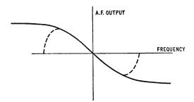
Fig. 7. A.F. output against frequency for gated-beam discriminator, assuming limiting at all frequencies. The dotted curve is that obtained in practice due to falling-off of signal amplitude with circuit selectivity.
