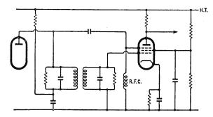
Fig. 4. Circuit for use with gated-beam discriminator.
