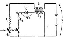
Fig. 6. The blocking oscillator circuit (Fig. 1) can be simulated quite well during its trigger phase by this working model, in which the value is represented by  $R_1$ ,  $R_2$  and the two-pole switch.
