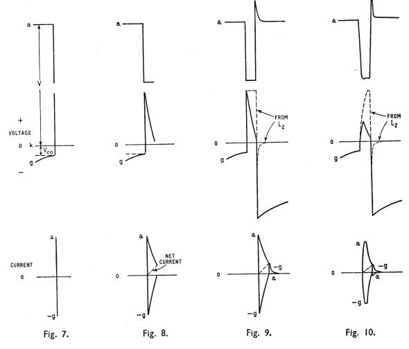
Fig. 7. First stage of the continuation of Fig. 3: the trigger action " on."
