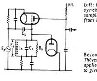
Left: Fig. 11. Circuit of synchrotector with sampling pulses derived from input signal.
