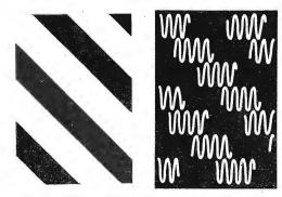
Fig. 4. When scanning diagonal bars (left) ordinary spot wobble gives a stepped effect (centre) but synchronous spot wobble fills in the spaces with genuine picture information (right).
