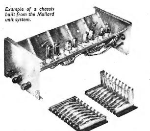
Carr Fastener printedcircuit connectors.
