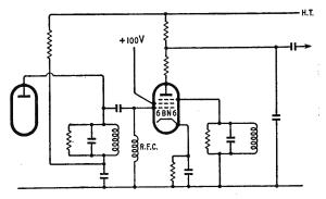
Fig. 8. Circuit used with 6BN6 gated-beam discriminator.
