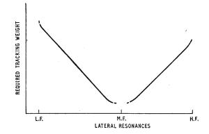
Fig. 5. Effect of lateral resonances on required trucking weight.
