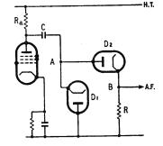
Right: Fig. 14. Basic " counter " circuit.
