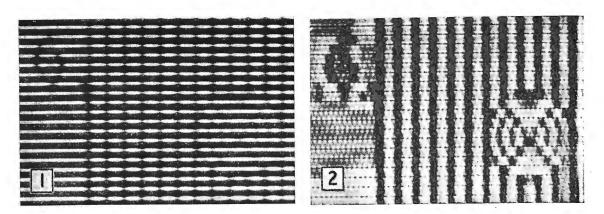
Fig. 1 shows a section of a test chart on one frame of a 405-line picture  $(202\frac{1}{2} \text{ lines})$  without spot wobble. Fig. 2 is the same section with ordinary spot wobble applied to the c.r.t., while Fig.3 (on opposite page) shows the improvement effected by synchronous spot wobble on both c.r.t. and camera tube. A complete interlaced picture with s.s.w. is even better.
