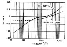
Fig. 7. Suggested revision of recording characteristics.
